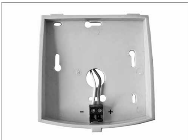
Fig. 28: Connect the room controller
