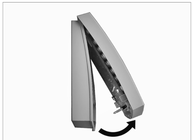
Fig. 27: Opening the housing
