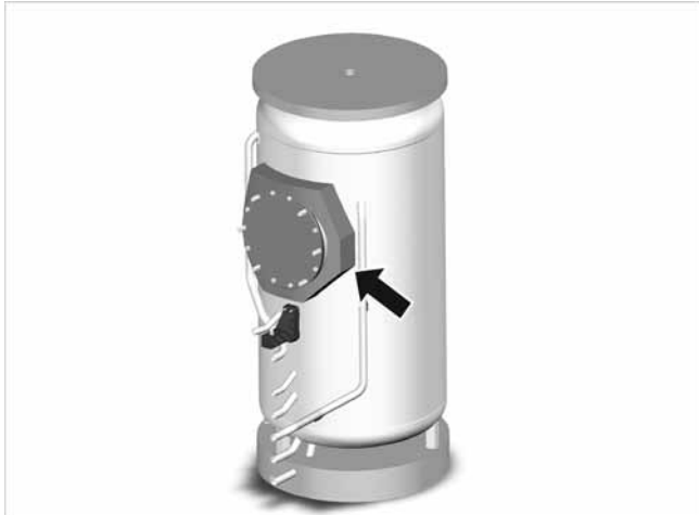
Fig.5: Fit the flange collar shell
