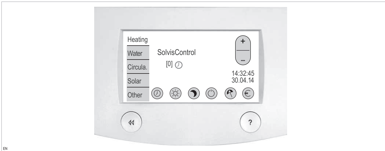
Fig. 5: SolvisControl with "Heating" menu
